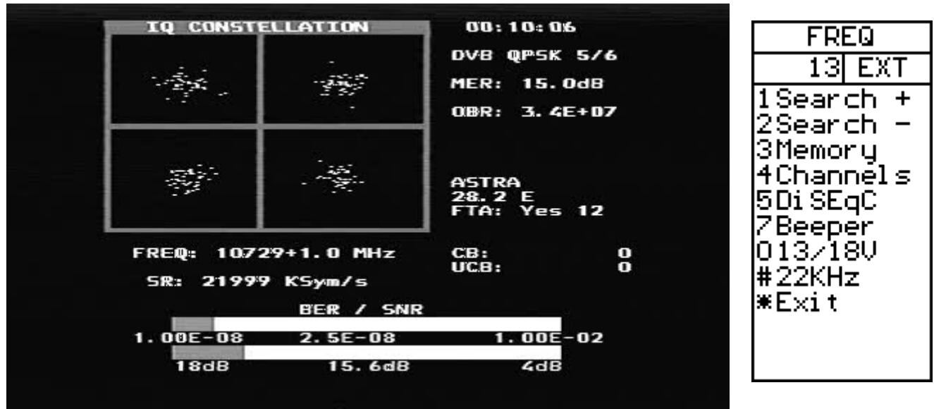
**Search +/-)** A signal search can be initiated by using the keypad '1 Search +' to search with increasing frequency or '2 Search -' with decreasing frequency. The search mode moves to the next peak in the spectrum and attempts a lock for DVB-S QPSK, DVB-S2 QPSK and DVB-S2 8PSK signals. The symbol rate is determined automatically. Because the time to lock for low symbol rate signals increases the lower the symbol rate, symbol rate signals below about 16000 will not lock during a search.
