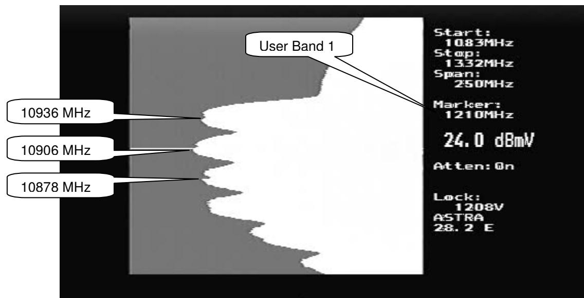
The UniCable test (Spec -> UniCable -> Uni Test) allows full testing of a UniCable LNB. This test takes about 20 seconds to check each User Band. During the test, the four User Bands are identified and any offset found is used for further UniCable tuning.
