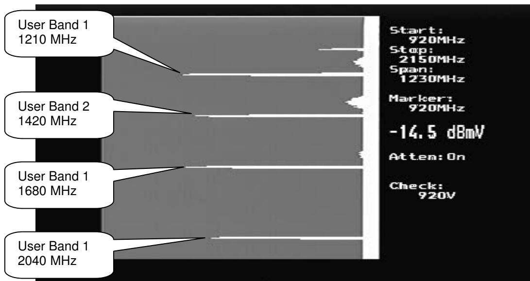
At the end of the test, the results of measuring the User Bands are presented.
