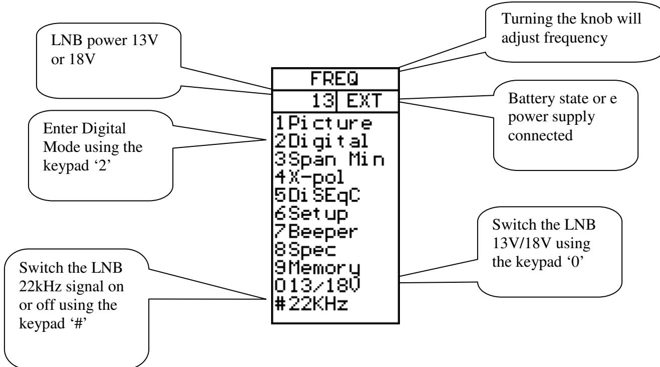
When the operation can use a memory location, the lower portion of the LCD shows the current memory selection. For this case, the knob is used to change the memory position number that the 'Save' will use.
