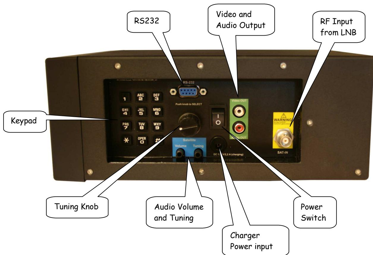
**Power Switch)** On battery power, this turns the instrument on and off. When the charger is connected, the instrument will charge with the switch off, and operate when on. The instrument will not charge when operating.
